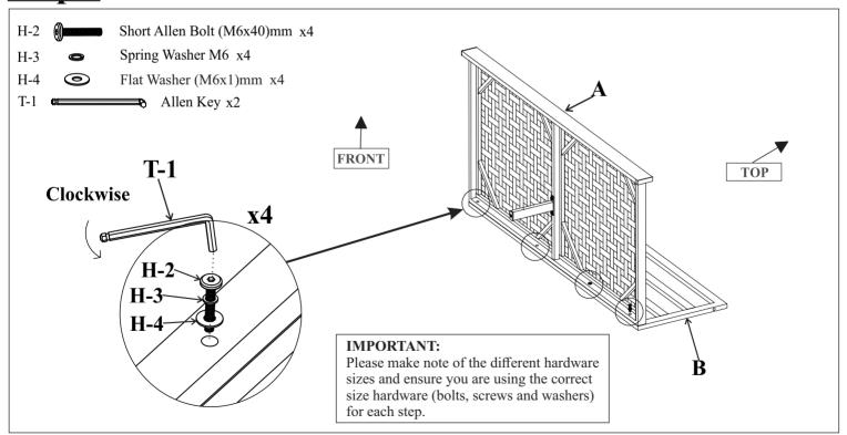
Using a second person to assist you, position the Seat Frame (A) with the Back Frame (B) as shown. While one person holds the Seat Frame (A), secure with Short Allen Bolts (H-2), Spring Washers (H-3) and Flat Washers (H-4) using the provided Allen Key (T-1), stacking the hardware in the order as shown. Engage all bolts first, then fully tighten. DO NOT OVER TIGHTEN.
