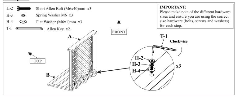
Using a second person to assist you, position the Seat Frame (A) with the Back Frame (B) as shown. While one person holds the Seat Frame (A), secure with Short Allen Bolts (H-2), Spring Washers (H-3) and Flat Washers (H-4) using the provided Allen Key (T-1), stacking the hardware in the order as shown. Engage all bolts first, then fully tighten. DO NOT OVER TIGHTEN.
