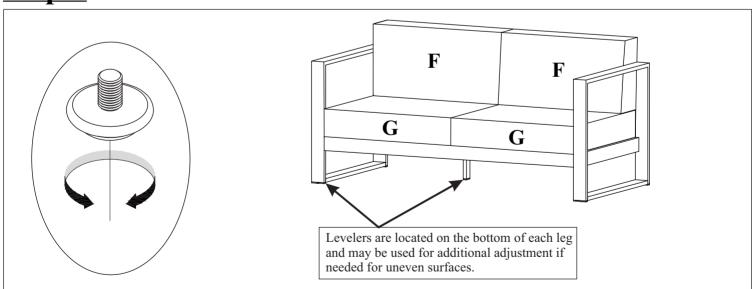
Using a second person to assit you, turn the assembly upright. Place Seat Cushions (G) and Back Cushions (F) into position as shown above. Ensure the zippers face down.
