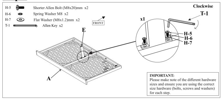
Using a second person to assist you, Place Seat Frame (A) upside down onto a padded, non-marring surface. Position the Center Leg (E) onto the crossbars as shown. Secure both Center Leg (E) to the Seat Frame (A) with Shorter Allen Bolts (H-5), Spring Washers (H-6) and Flat Washers (H-7) using the provided Allen Key (T-1), stacking the hardware in the order as shown. Engage all bolts first, then fully tighten. DO NOT OVER TIGHTEN.
